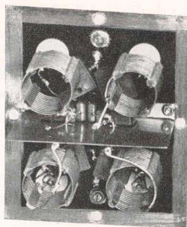
Fig. 2. Detail views of a 3.5-megacycle, 300-ohm balanced type Harmoniker. Ground posts G and G' are located between each pair of coils, which are supported by their leads.
